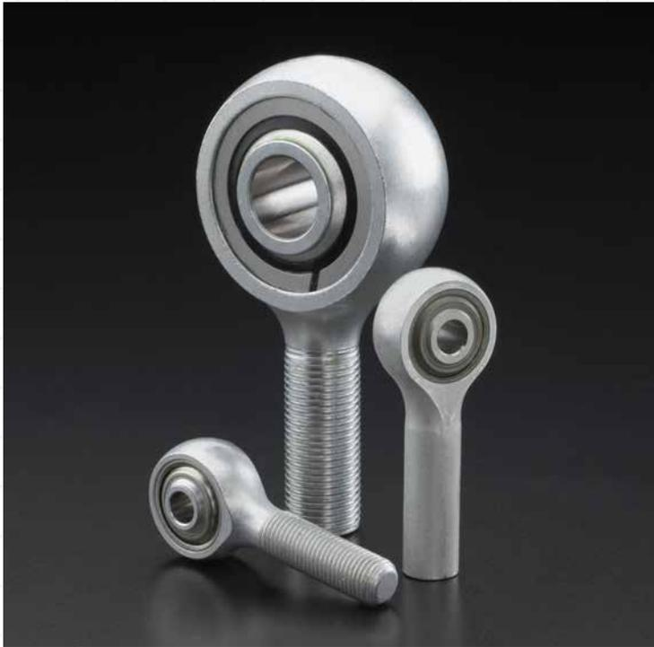
**Heim<sup>®</sup> AeroCres<sup>®</sup> Ball Bearing Rod Ends** are precision ground to tight tolerances for applications requiring self alignment, low torque and reduced radial clearance. They are greased and equipped with PTFE seals bonded to corrosion resistant caps.
