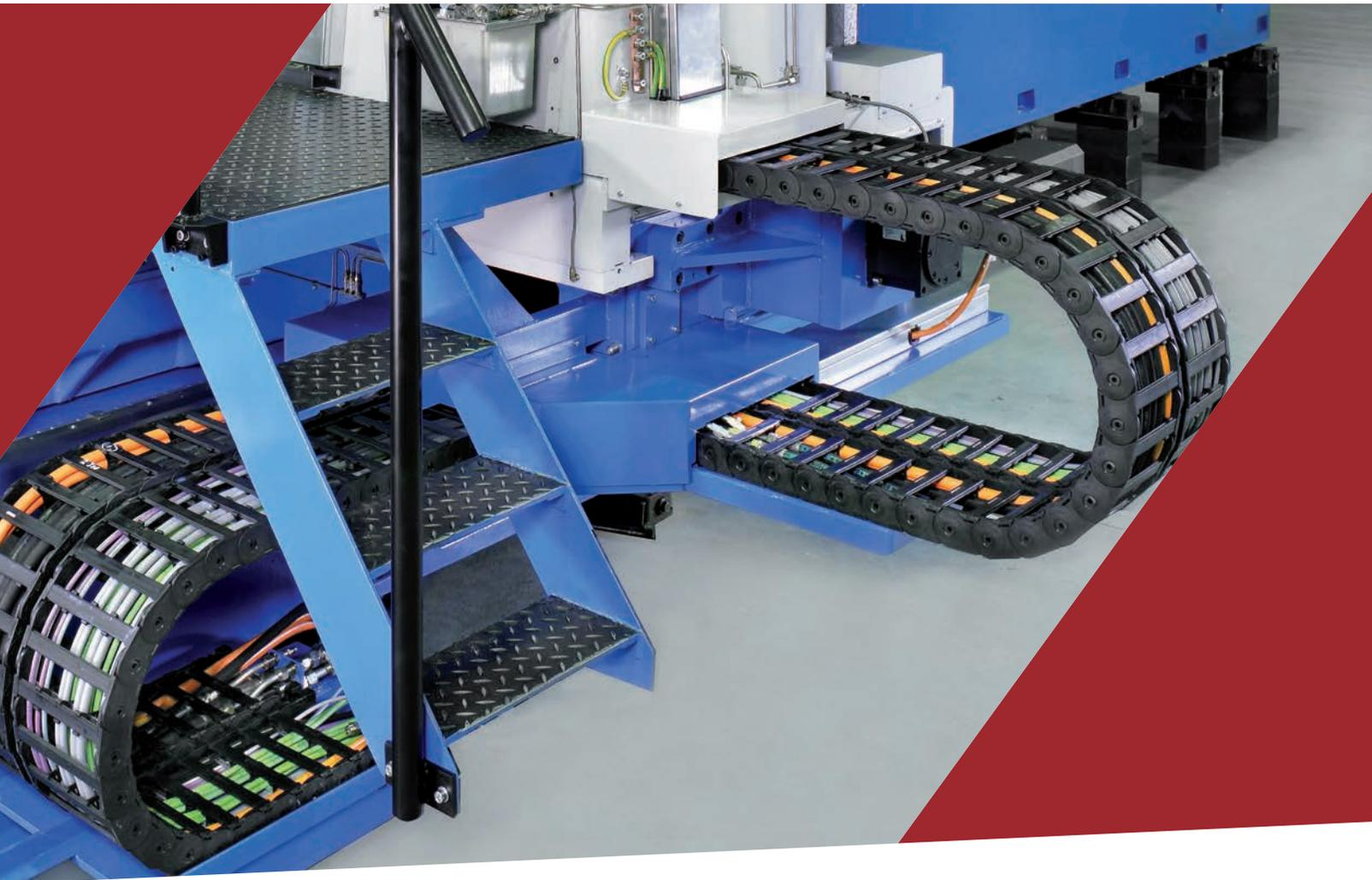
Our basic program includes different product types with simple design and predefined chain widths. All product types combine robustness and reliability with an excellent price-performance ratio. Cables can be quickly and easily installed into these carriers. Covered and fully enclosed product types guarantee optimum protection of cables and hoses against chips and other coarse dirt.
