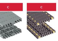
PSX 1001 Series HP 8506 Series MTW PT MTW PT PITCH: 1-inch PITCH: 3/4-inch (25.4mm) (19.05r HEIGHT: 0.35-inch HEIGHT: 0.35-inch (8.7mm) (8.7mm) For high-speed single For high-speed single file conveyors; vacuum file conveyors and holes optional magnetic elevators
