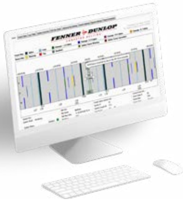
Splice, damage and rip detection events are actively tracked as the conveyor stops.
