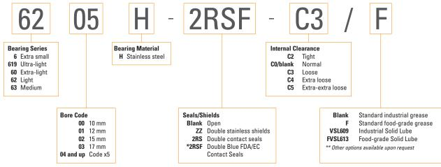
\*Complies with FDA guidelines for indirect food additives under 21 CFR 177.2600 'Rubber articles intended for repeated use', and meets the requirements of EC 1935/2004 'materials and articles intended to come into contact with food'.
