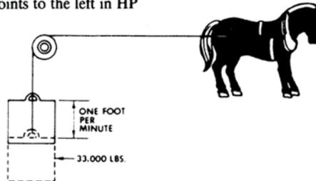
$$\begin{aligned} \text{HP} &= \frac{\text{Force} \times \text{FPM}}{33,000} \\ \text{HP} &= \frac{\text{Torque (in Pound-Inches)} \times \text{RPM}}{63,025} \\ \text{HP} &= \frac{\text{Torque (in Pound-Feet)} \times \text{RPM}}{5,252} \end{aligned}$$
