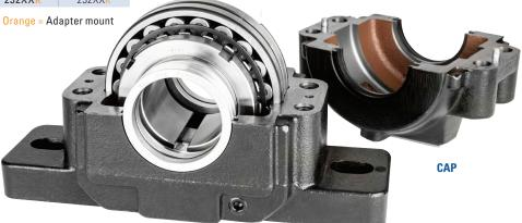
Mounted bearings are also called "pillow blocks" (inch) or "plummer blocks" (metric). The SAF mounted spherical roller bearings are typically easy to install by securing the base, installing the spherical roller bearing and adding lubricant, then aligning the matching cap in place with the dowels. Caps and bases are manufactured as a matched set for a precision fit.
