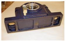
Rugged Base Provides for Superior Housing Strength and Allows for Oil Equalization Slots Under Bearing Seat. This Ensures a Balanced Oil Level on Each Side of the Bearing.
