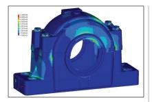
Among the Heaviest in the Industry, PTI SAF Housings Were Designed Using Finite Element Analysis (FEA).
