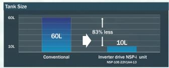
The NSP-i series benefits your entire system by lowering oil temperature to improve machining accuracy, lengthen the life of seals and hydraulic fluid, and reduce factory air conditioning costs.
